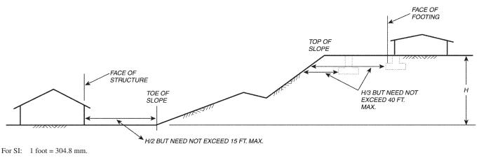
FIGURE 1805.3.1 FOUNDATION CLEARANCES FROM SLOPES
